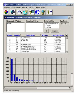
Figure 2 - Example of failure rate evaluation
